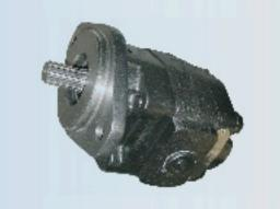
The P22 direct gear pump is bi-rotational with side and rear ports for versatility, thus eliminating the drive line for added safety and dependability. This pump has an S.A.E. "B" 2-bolt flang. 15 GPM @1200 RPM
